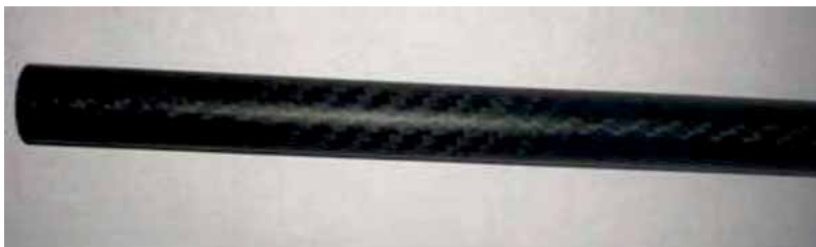
Development of Carbon Fibre Tue used in Drone Assembly - M/s. Eagle eye Drones, Mysuru; by CIPET: CSTS, Mysuru
